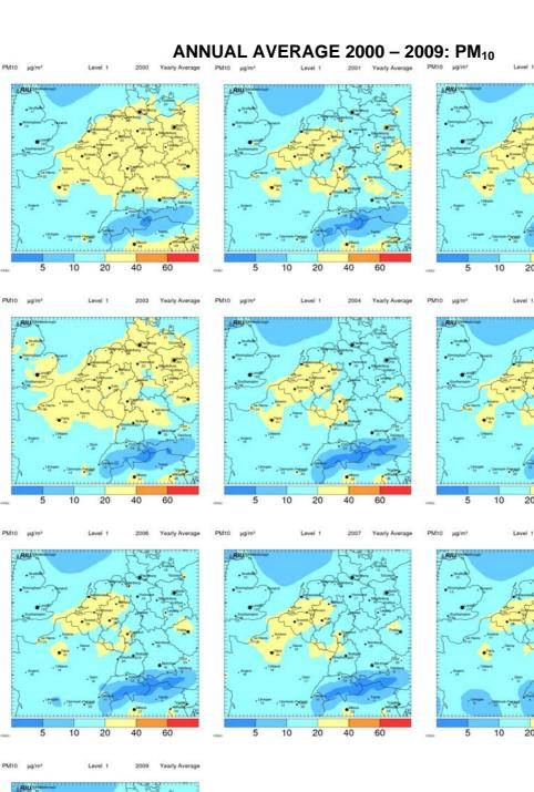
Figure 2b: Annual average of  $PM_{10}$  for the N1-domain (25 km grid size, see Figure 1) for the year 2000 till 2009. Data are calculated on the basis of hourly values.
