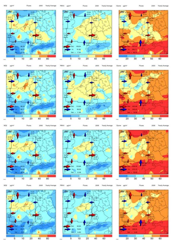
Figure 3d: Budget calculations for NO<sub>2</sub>, PM<sub>10</sub> and O<sub>3</sub> for the enlarged Benelux-Rhine-Ruhr area as indicated in the figure for 2000 – 2009. The calculations are performed up to a height of 2500 m. Fluxes are given in  $\mu$ g/m<sup>2</sup>s.
